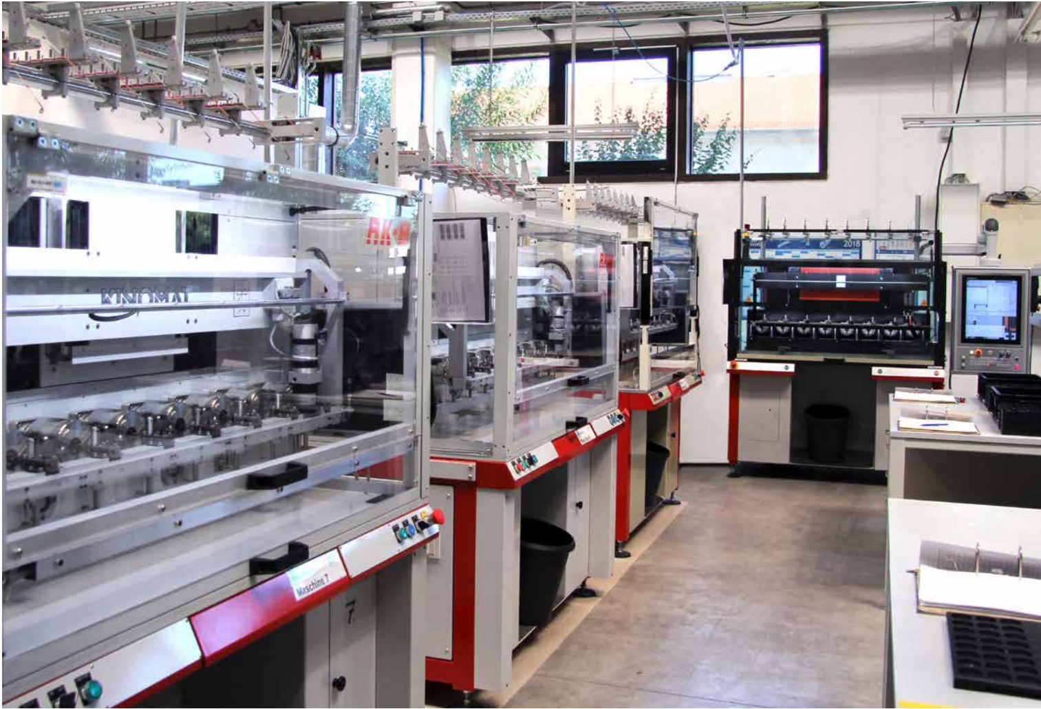
The upgraded resolver winding machine with TNC 620 control is located at the head end, with three of the six systems to be retrofitted by the end of 2019 on the left.
