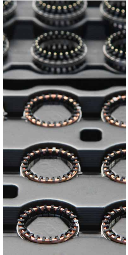
Before and after: Finished stator winding cores below and empty ones above.
