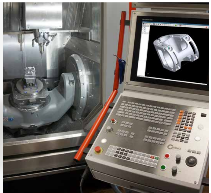
The 3-D data of a complex component, for example this mountain bike handlebar mount, can be directly loaded into the NC program.
