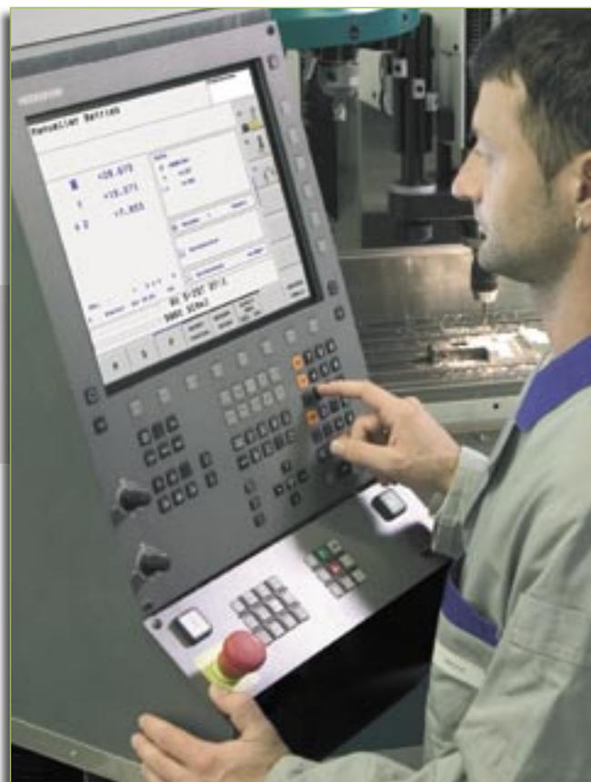
In order to keep set-up times as brief as possible, field-proven probing cycles are available in the Manual operating mode for you to quickly and accurately ascertain workpiece locations and orientations, as well as set reference points.
