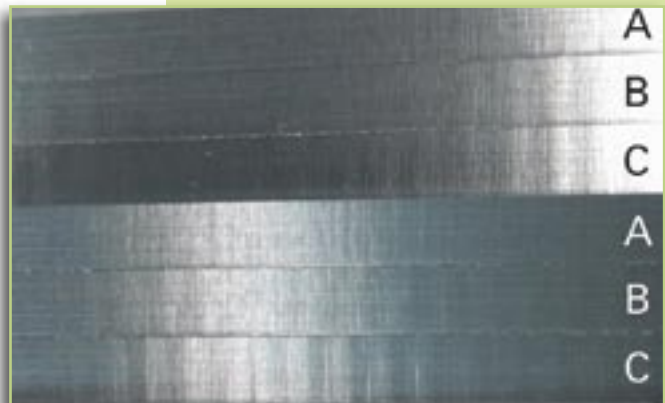
Quality of a milled workpiece surface manufactured with different degrees of signal quality.
