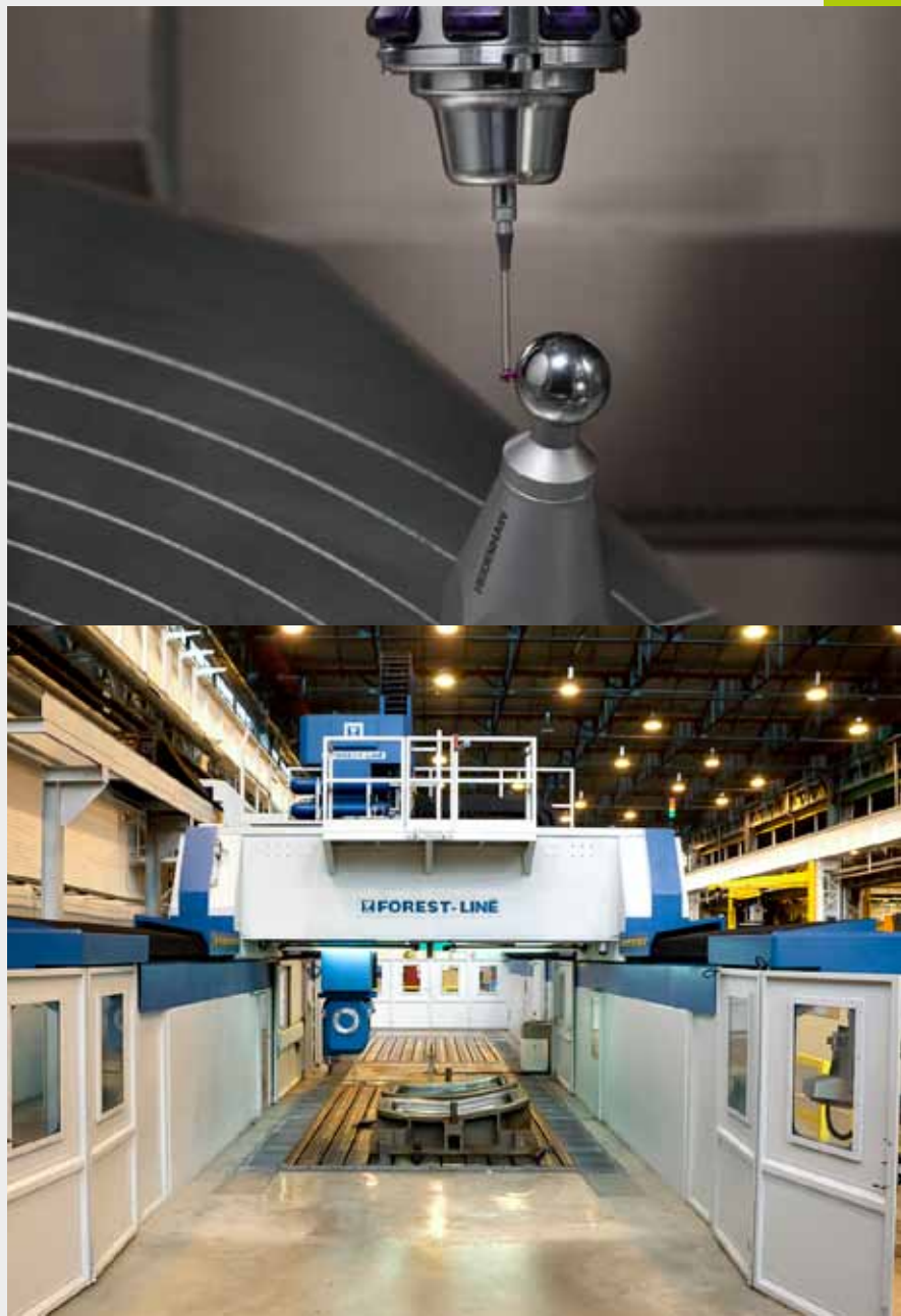
Reproducible tilting accuracy over long periods with KinematicsOpt.
