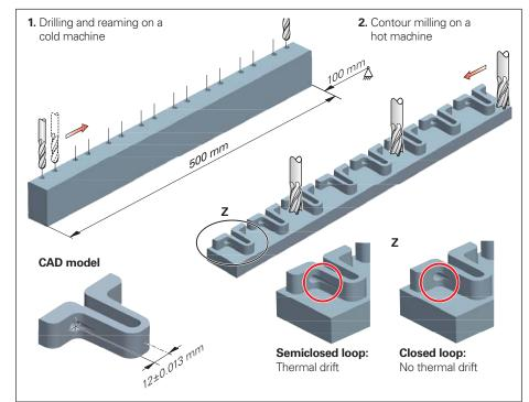
Figure 3 Effect of drive accuracy on the production of small parts  $\Delta =$  Fixed bearing of the recirculating ball screw
