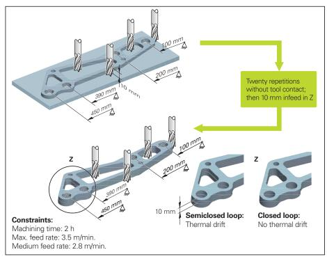
Figure 5 Manufacturing of the coupling lever  $\hat{\mathbf{A}} = \text{Fixed bearing of the recirculating ball screw}$
