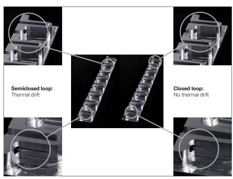
Figure 4 Effect of drive accuracy on the series production of small parts
