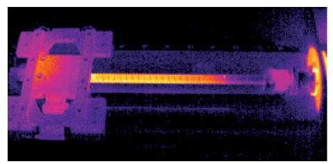
Figure 1 Heating of a recirculating ball screw during multipass milling at a mean feed rate of 10 m/min. This thermographic snapshot shows temperatures of 25 °C I to 40 °C I.
