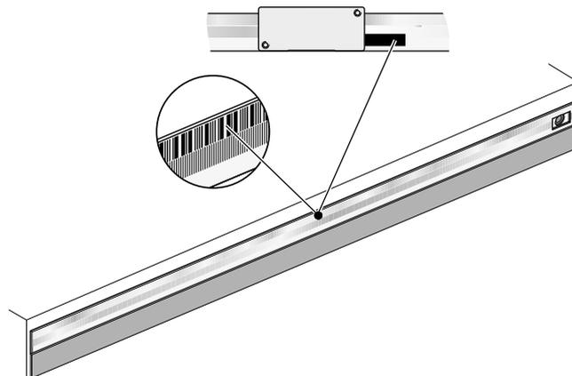
The scale tape with the PRECIMET adhesive mounting film has to be attached at a temperature > 15 °C! Pay attention to the expiration date on the package! Peel off the mounting film's protective film around the punched hole as shown; protect the adhesive surface from contamination!
