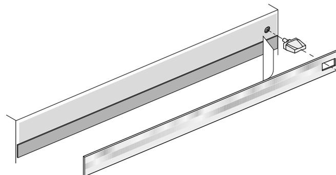
Starting from the middle, press the scale tape evenly onto the mounting surface using a roller.
