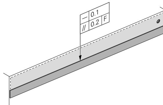
Use the mounting aid to align the scale tape, and gently glue it along the aligning rail.
