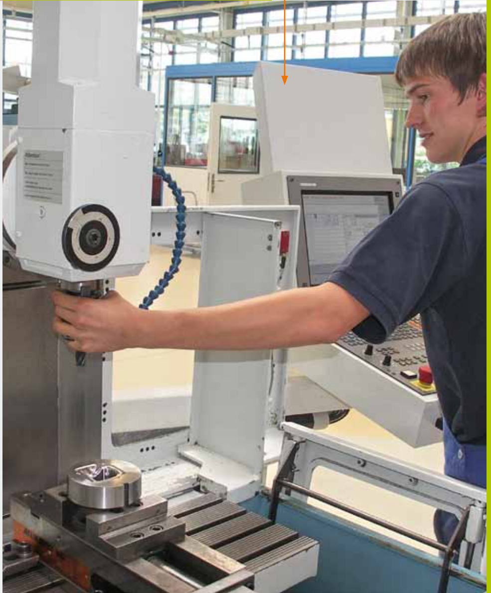
Christian Maisson, apprentice on a Maho 400E milling machine that he personally retrofitted to its HEIDENHAIN control
