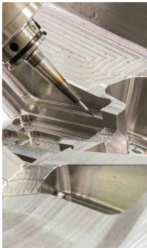
The Müller Modell- und Formenbau company produces complex tools for the injection molding of plastic automotive parts with the iTNC 530—see page 12 for details
