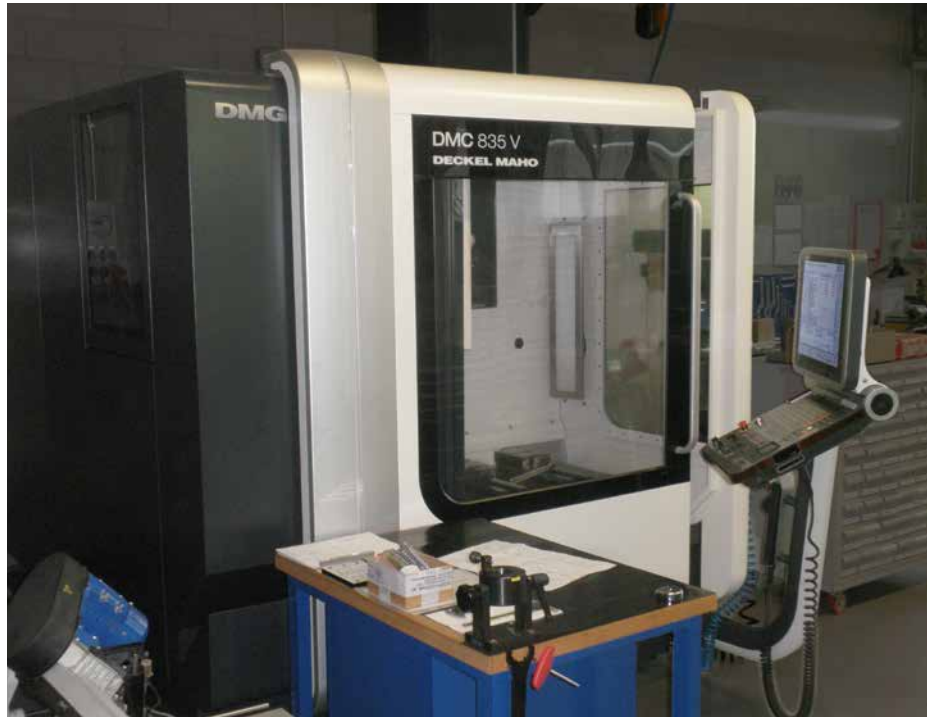
NC programs are created directly on the TNC controls to enable components to be flexibly and rapidly produced with turning, drilling and milling cycles.
