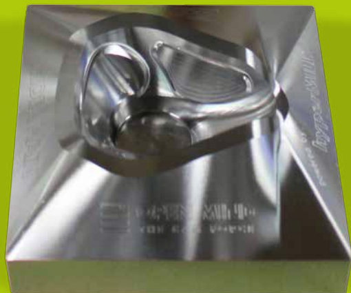
In the workshop the form for a respiration mask was machined with the iTNC 530 HSCI. A challenge was the material itself: A corrosion-resistant plastic mold steel 1.2083.
