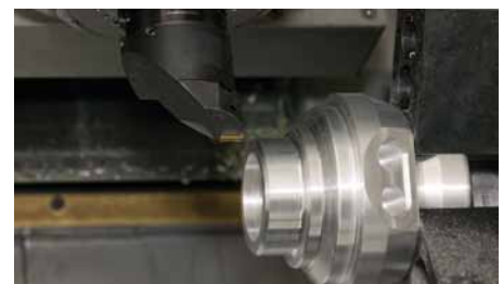
... longitudinal turning with the same tool.
