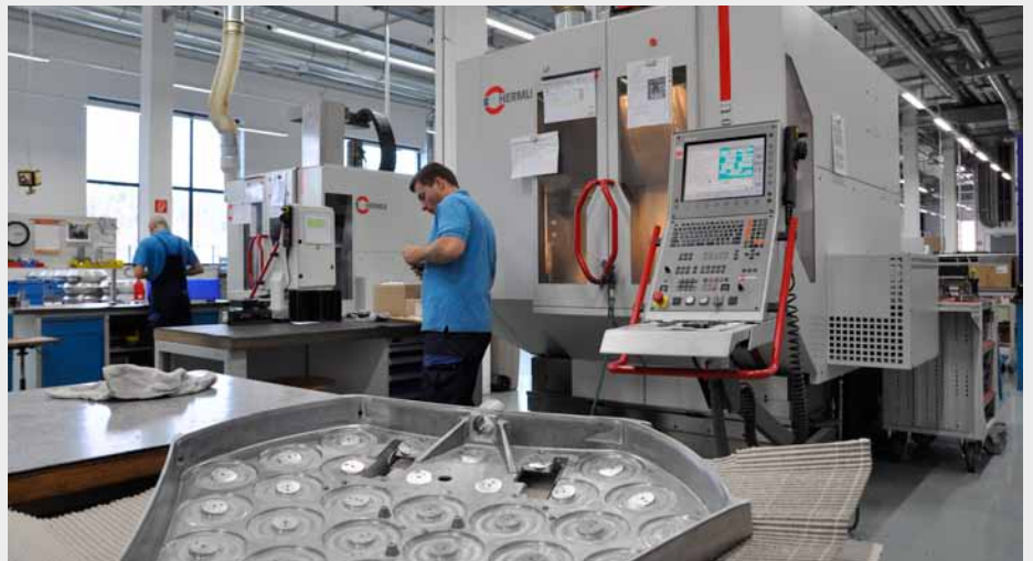
The casting is machined in only one setup.
