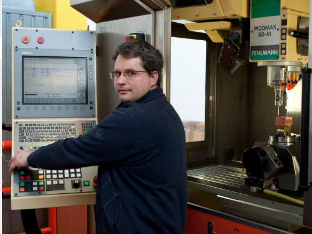
The iTNC 530 during sample production—simple conversational programming for complex operations
