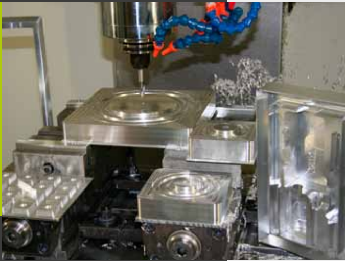
With the HEIDENHAIN TNC 620, three-axis machining is realized simply and effectively.
