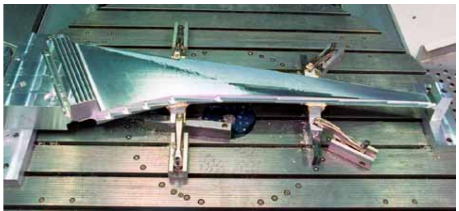
Airplane wing of a wind-tunnel model, which can consist of up to 800 parts.
