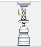
Measuring the tool length with stationary or rotating spindle
