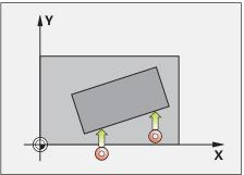
Measuring the angle of a line
