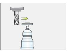
Measuring the tool radius with rotating spindle
