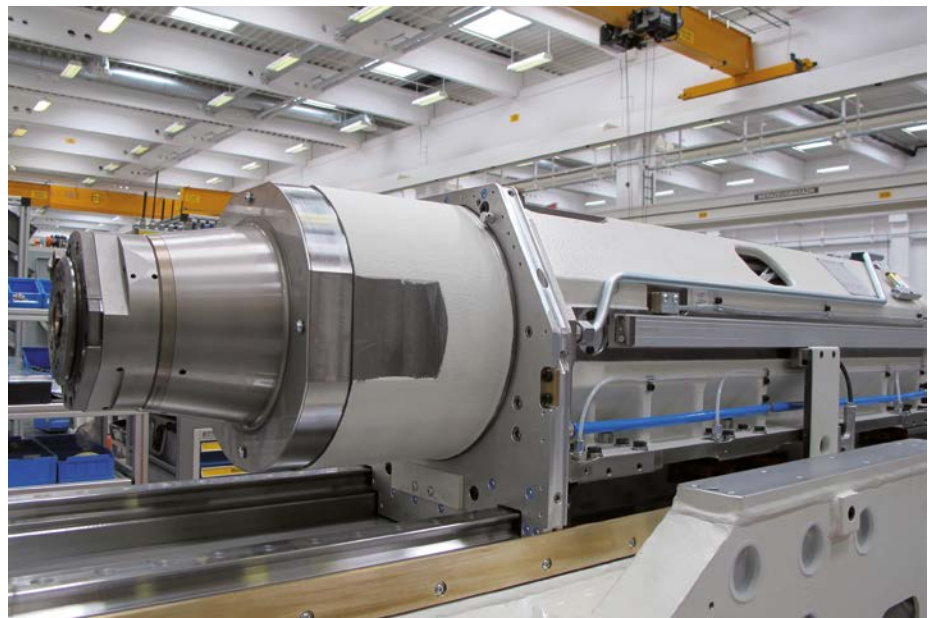
Figure 5: HEIDENHAIN linear encoder in a horizontal machining center (photo: GROB-WERKE GmbH & Co. KG)
